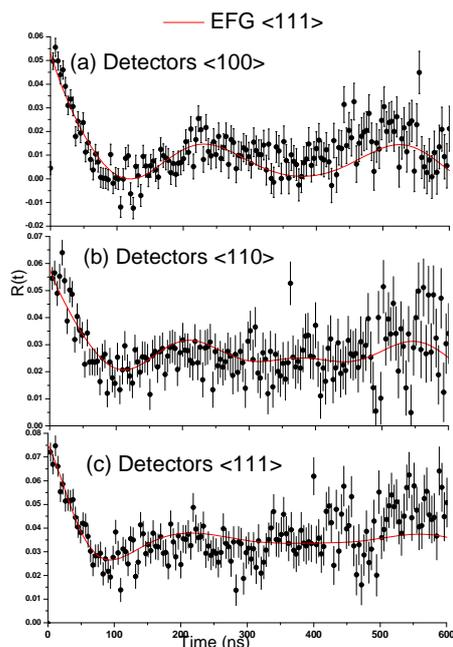
Fig. 4. Measured ratio functions  $R(t)$  for  $^{100}\text{Pd}/^{100}\text{Rh}$  in germanium for the three specimen orientations. The data are compared with a calculation that assumes that about 25% of the palladium probe atoms pair with vacancies and that the defect pair and EFG are oriented in the  $\langle 111 \rangle$  direction.
