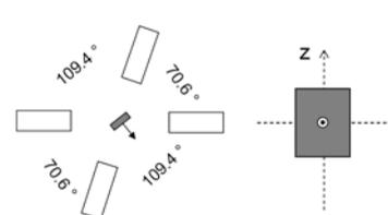
Fig. 2. Respective orientations of the detector array and the germanium specimen (grey). The arrow points in the  $\langle 100 \rangle$  direction.
