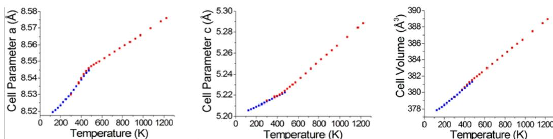
Fig. 3. Unit cell parameters a, c and cell volume as the temperature of Ba<sub>2</sub>TiSi<sub>2</sub>O<sub>8</sub> is increased from 125 K to 1223 K. Blue and red data points indicate data collected using a low-temperature and high temperature attachment, respectively.
