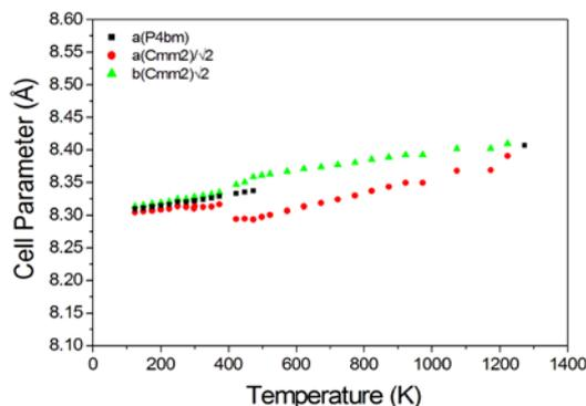
Fig 4: The change in unit cell parameters a and b in the *Cmm2* phase (red and green, respectively) overlaid with unit cell parameter a for the *P4bm* phase (black) between 125 - 1273 K.
