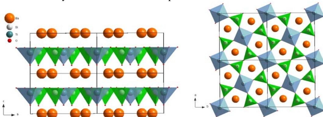
Fig 1. The fresnoite  $\text{Ba}_2\text{TiSi}_2\text{O}_8$  structure projected along the  $a$  (left) and  $c$  (right) directions. The large barium cations exist in cavities formed between  $(001)$  sheets of corner-linked  $\text{TiO}_5$  and  $\text{SiO}_4$  polyhedra.
