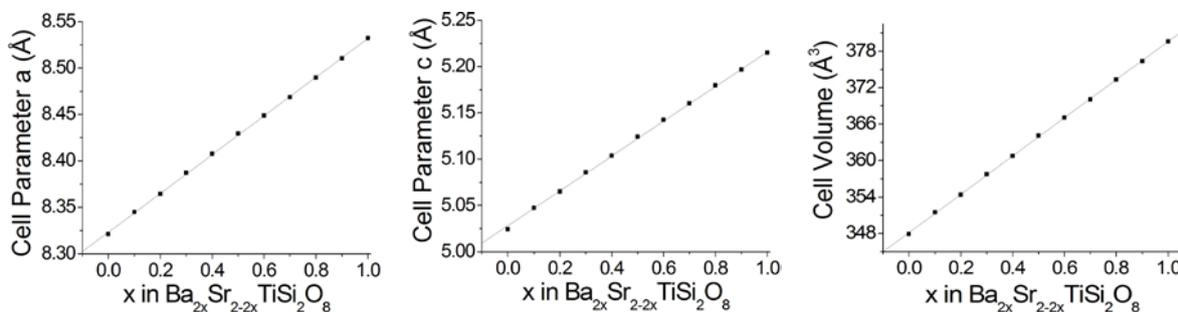
Fig. 2. Unit cell parameters  $a$ ,  $c$  and unit cell volume as a function of composition for the series  $\text{Ba}_{2x}\text{Sr}_{2-2x}\text{TiSi}_2\text{O}_8$  ( $0.0 \leq x \leq 1.0$ ) at ambient temperature.
