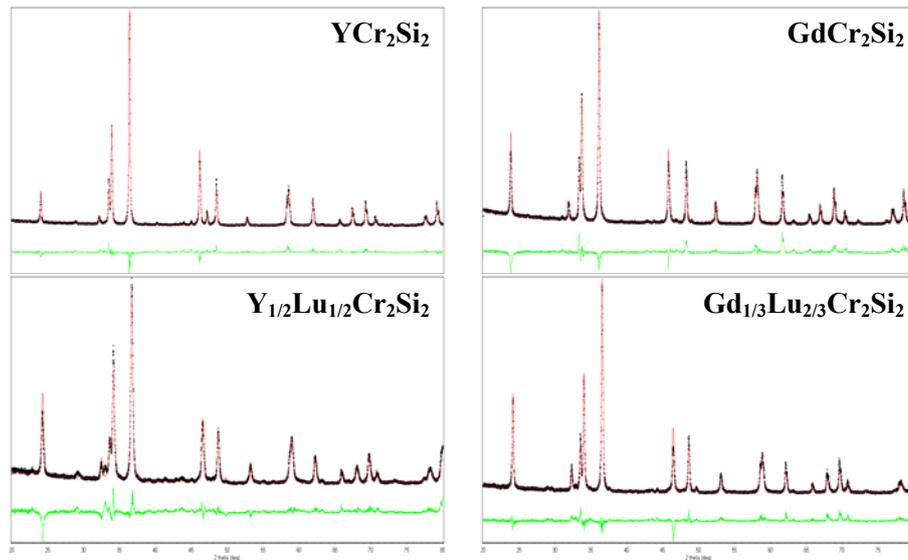
Fig. 1. X-ray diffraction patterns for  $\text{YCr}_2\text{Si}_2$ ,  $\text{Y}_{1/2}\text{Lu}_{1/2}\text{Cr}_2\text{Si}_2$ ,  $\text{GdCr}_2\text{Si}_2$  and  $\text{Gd}_{1/3}\text{Lu}_{2/3}\text{Cr}_2\text{Si}_2$ . The solid lines beneath the plots indicate the difference between the experimental data and the fitted Rietveld theory.
