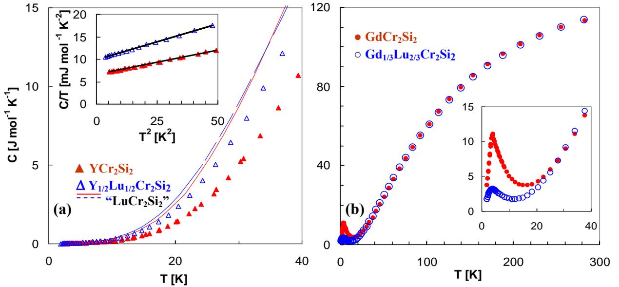
Fig. 2. Specific heat data for (a)  $\text{YCr}_2\text{Si}_2$  and  $\text{Y}_{1/2}\text{Lu}_{1/2}\text{Cr}_2\text{Si}_2$  and (b)  $\text{GdCr}_2\text{Si}_2$  and  $\text{Gd}_{1/3}\text{Lu}_{2/3}\text{Cr}_2\text{Si}_2$
