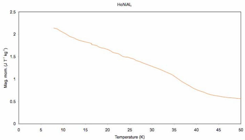
Fig. 3. Magnetisation data for polycrystalline HoNiAl<sub>4</sub>.
