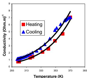
**Figure 1.** Temperature dependence of conductivity of a C<sub>60</sub> film in vacuum 10<sup>-7</sup> Torr after one heating/cooling cycle.
