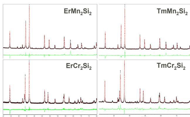
Fig. 1. X-ray diffraction patterns for  $\text{ErMn}_2\text{Si}_2$ ,  $\text{ErCr}_2\text{Si}_2$ ,  $\text{TmMn}_2\text{Si}_2$  and  $\text{TmCr}_2\text{Si}_2$
