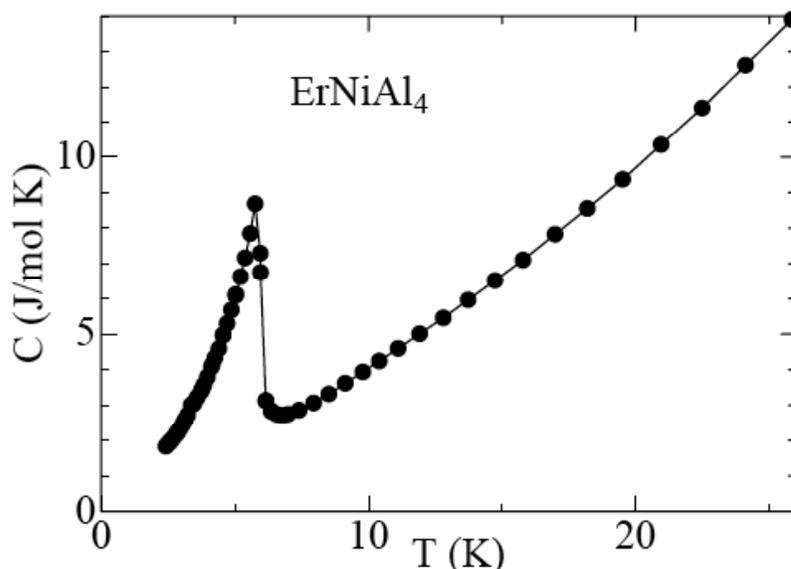
Fig. 1. Specific heat measurement for ErNiAl<sub>4</sub> in zero magnetic field.
