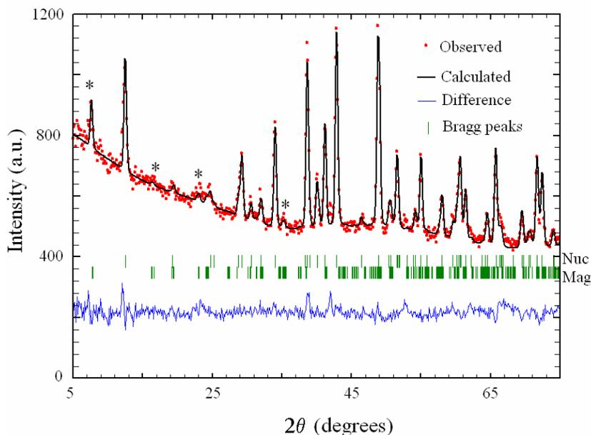
Fig. 3. Neutron diffraction data for  $\text{ErNiAl}_4$  powder, collected in zero applied magnetic field and at a sample temperature close to 5.8 K. The Fullprof refinement suggests incommensurate magnetic order (starred peaks).
