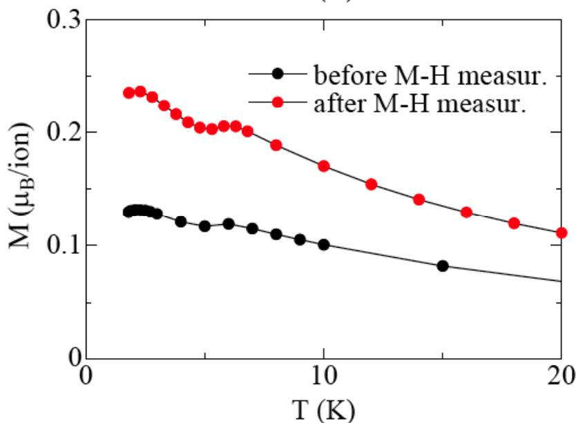
Fig. 2. Magnetisation measurements for ErNiAl<sub>4</sub> powder, collected at 0.1 T applied magnetic field, before and after exposing the sample to a high magnetic field (7 T).
