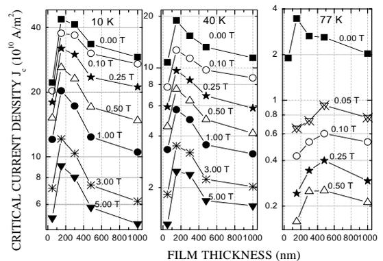
Fig. 3.  $J_c(d_p)$  dependencies at different fields and temperatures for YBCO films deposited at 6Hz.
