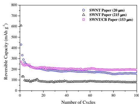
Fig. 4. Reversible capacities vs. cycle number. The current density was  $0.08 \text{ mA cm}^{-2}$ .
