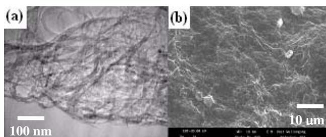
Fig. 2. (a) TEM image of SWNTs precursors; and (b) typical SEM image of SWNT paper.
