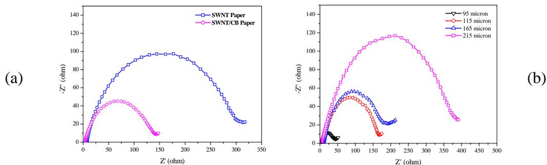
Fig. 3. Nyquist plots for (a) SWNT paper and SWNT/CB composite paper, and (b) SWNT paper with different thicknesses.
