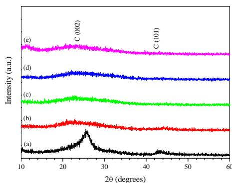
Fig. 1. XRD patterns of (a) carbon black powder, (b) SWNTs precursors, (c) thin SWNT paper with thickness of 30  $\mu\text{m}$ , (d) SWNT paper with thickness of 180  $\mu\text{m}$  and (e) SWNT/CB composite paper with thickness of 120  $\mu\text{m}$ .
