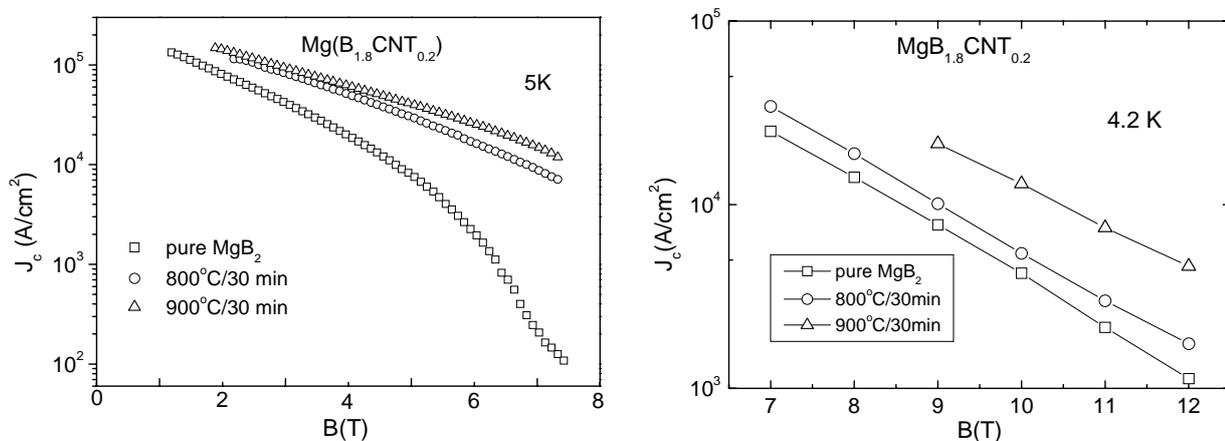
Fig.3: Magnetic (a) and transport (b)  $J_c$  for carbon-nanotube doped  $MgB_2$  sintered at different temperatures.
