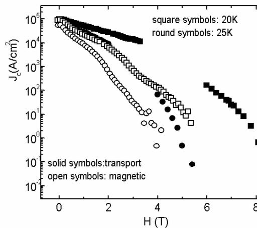
Fig.2: Transport and magnetic  $J_c$  for Cu-sheathed  $MgB_2$  wire .
