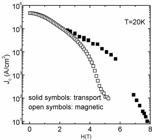
Fig.1: Transport and magnetic  $J_c$  for Fe-sheathed  $MgB_2$  wire.
