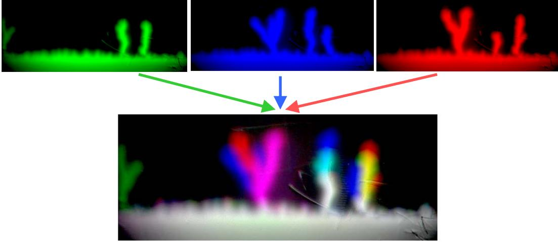
Fig. 2. (top) Magneto-optical images of flux penetration in 3 experiments under identical external conditions. (bottom) A sum image of the 3 images above. Overlap of colored regions in all 3 images appears as white, whereas no or only partial overlap appears as another color.
