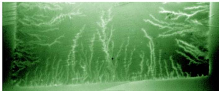
Fig. 1. Magneto-optical image of dendritic flux penetration in an MgB<sub>2</sub> film at 4 K. The brightness in the image represents the local flux density. The lateral size of the sample is  $2w = 4$  mm.
