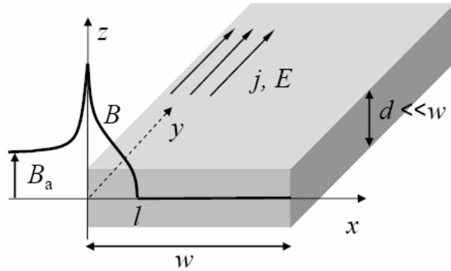
Fig. 3. Schematic of fields and currents in a long thin superconducting strip during ramping up of a perpendicular applied magnetic field. Only the left half of the strip is shown.
