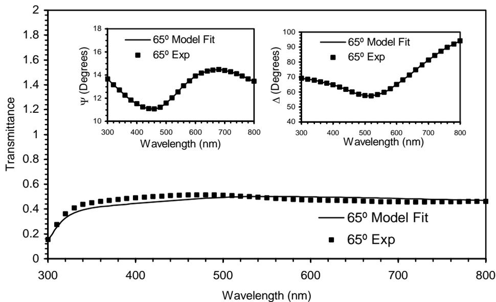
Figure 2: Main plot is spectrophotometric transmittance. Inset plots are ellipsometric data  $\psi$  and  $\Delta$  ( All data was obtained at 65° incidence angle for a 20nm spongy nanoporous gold film on glass.
