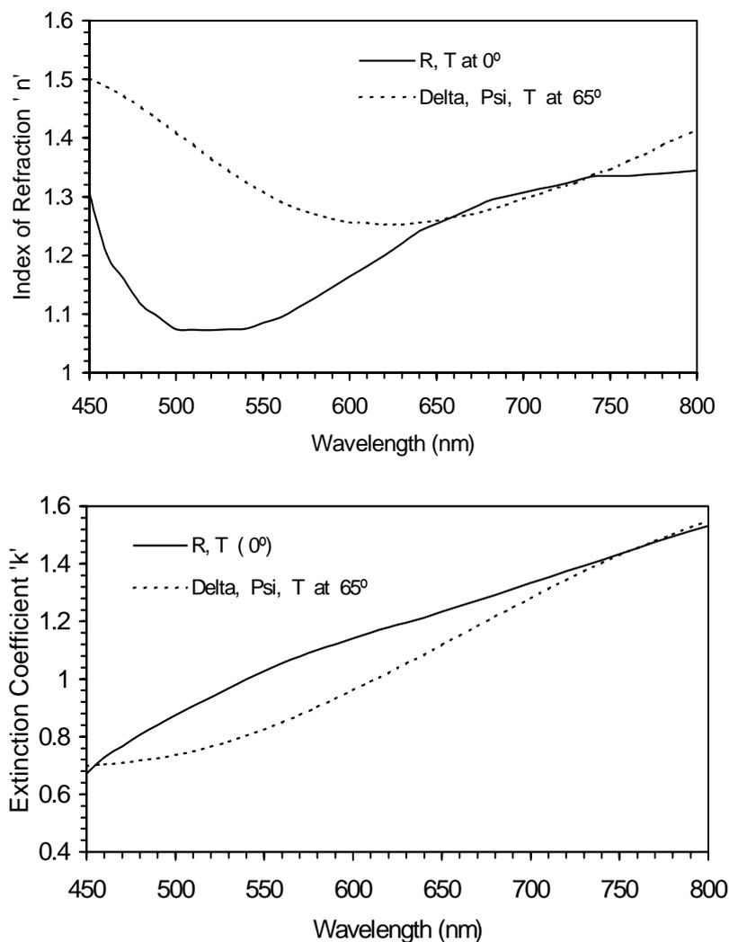
Figure 3: Optical constants ( $n^*$ ) and ( $k^*$ ) as a function of wavelength and angle of incidence for a 20nm spongy nanoporous gold film on a glass substrate obtained from the fit of ellipsometric data ( $\Delta$ ,  $\Psi$ ) combined with spectroscopic transmittance at  $65^\circ$  (dotted line) and transmittance and reflectance at  $0^\circ$  (solid line).
