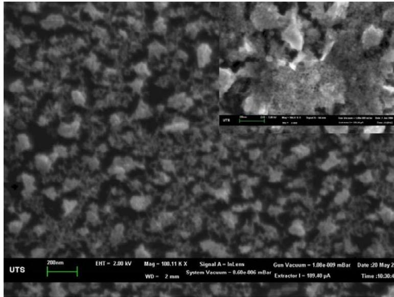
Figure 1: SEM image of the 20nm spongy nanoporous gold film taken at magnification X100000 while the inset image is at X188000.
