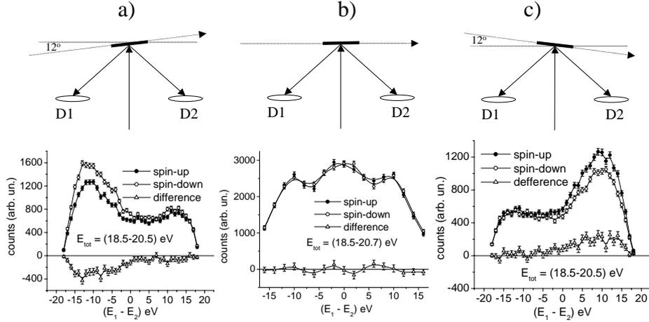
Figure 4: Energy sharing distributions of correlated electron pairs excited by 25.5 eV primary electrons from W(110) at three different positions of the sample.
