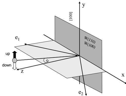
Figure 1: Geometry of the experiment, showing scattering plane as the ZX plane.
