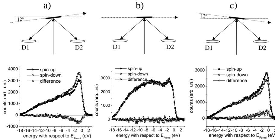
Figure 3: Binding energy spectra of W(110) recorded at three positions of the sample and primary electron energy 25.5 eV.
