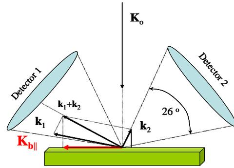
Figure 2: Momentum diagram of incident ( $K_0$ ), first ( $K_1$ ), second ( $K_2$ ) and valence ( $K_b$ ) electrons
