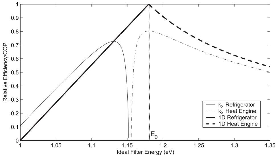
Figure 1: Heat-engine efficiency and refrigerator COP relative to the Carnot value for ideally filtered one-dimensional and  $k_x$  thermionic systems versus the energy of the ideal filter.
