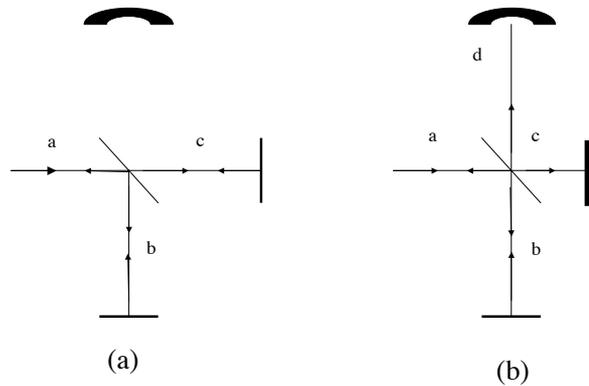
Figure 1: (a) Beam enters and exits on path  $a$  due to interference of reflected beams  $b$  and  $c$ . (b) Absorber on path  $c$  can lead to detection on path  $d$  of radiation that did not strike the absorber.
