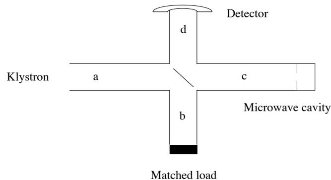
Figure 2: Conventional ESR spectrometer in schematic form.
