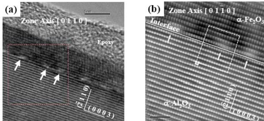
Figure 2: (a) HRTEM micrograph of the interface misfit dislocations imaged from the  $[01\bar{1}0]$  zone axis in which three misfit dislocations are present in the box marked by dashed lines. (b) The magnified and Fourier filtered image of the region in (a) showing an extra lattice plane in the  $\alpha\text{-Al}_2\text{O}_3$  side as indicated by the white arrow.
