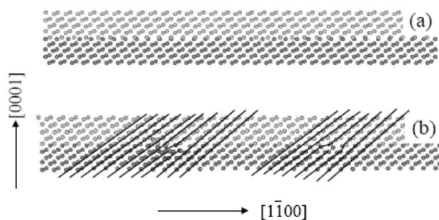
Figure 3: Atomic plots showing (a) the initial configuration of the interface along  $[1\bar{1}00]$  direction, when viewed from  $[11\bar{2}0]$  direction, and (b) the final configuration after relaxation. The solid lines are sketched to reveal extra lattice planes in the  $\alpha\text{-Al}_2\text{O}_3$  side.
