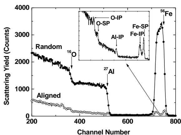
Figure 1: Aligned and random RBS spectra from epitaxially grown 70 nm thick  $\alpha$ -Fe<sub>2</sub>O<sub>3</sub> (0001) film on  $\alpha$ -Al<sub>2</sub>O<sub>3</sub> (0001) substrate. Incident energy of the He<sup>+</sup> was 2.04 MeV and the scattering was 150°. Magnified version of the aligned spectrum is presented in the insert.
