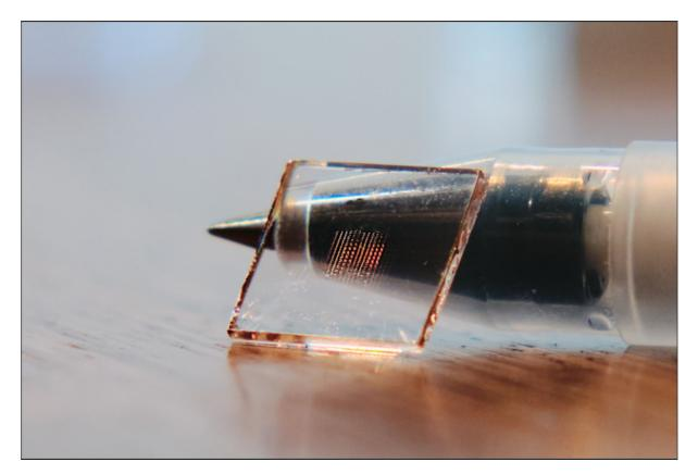
Structuring material on a nano-scale opens up great possibilities in modern photonics. While it is not possible to see by naked eye the actual design, the clusters of different meta-surfaces create beautiful diffraction patterns. Photo by Ivan Toftul.
