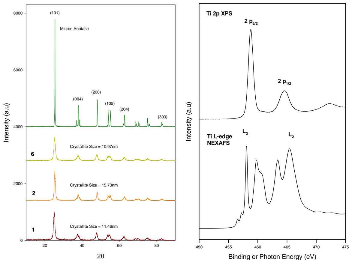
Figure 2 Left: Powder X-ray diffraction patterns for several  $\text{TiO}_2$  inverse opal powders and a micron sized anatase  $\text{TiO}_2$  powder. Right: Ti 2p XPS and Ti L-edge NEXAFS for a  $\text{TiO}_2$  inverse opal.
