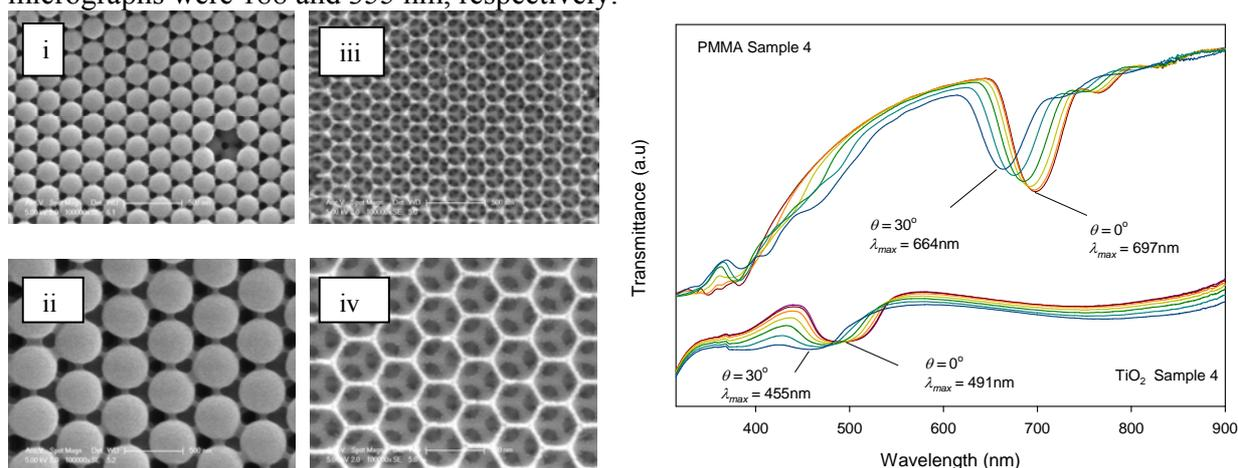
Figure 1(i) and (ii) show SEM micrographs for PMMA colloidal crystals of two different sizes. (iii) and (iv) show the corresponding TiO<sub>2</sub> inverse opals fabricated from the PMMA templates. The right panel shows UV-Visible transmission spectra for a PMMA colloidal crystal thin film (Sample 4) and its TiO<sub>2</sub> inverse opal replica. UV-Vis data were collected at angles of 0-30° with respect to the surface normal of the *fcc* (111) lattice planes.
