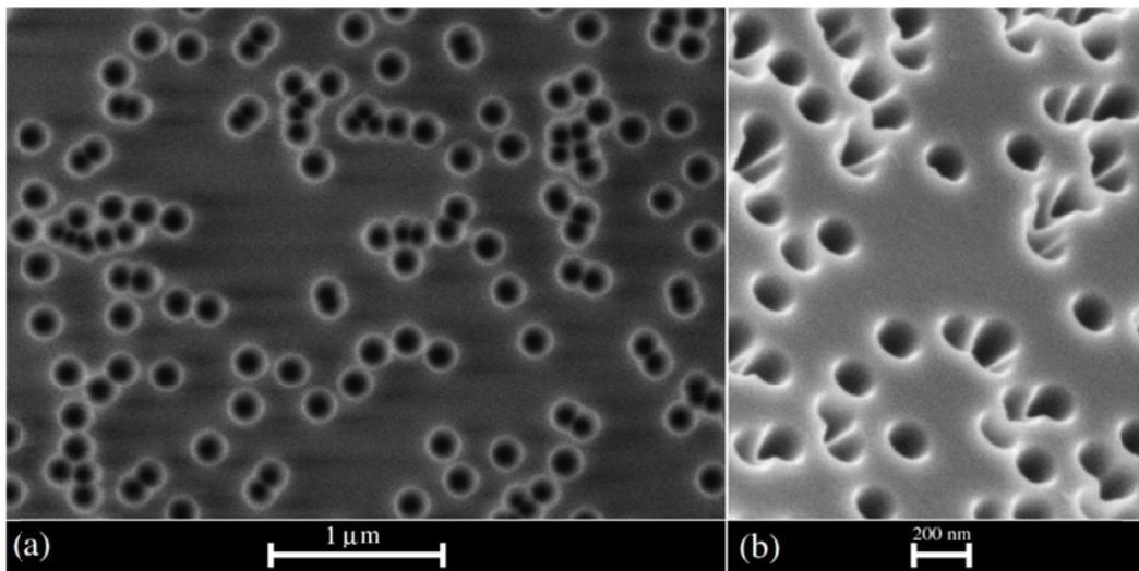
Fig. 1. (a) SEM top view image of etched ion tracks in a-SiO<sub>2</sub>, (b) SEM side view image
