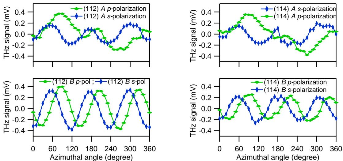
Fig. 2. Transmission geometry: Horizontal ( $p$ ) and vertical ( $s$ ) polarization components for GaAs (112) A, (112) B, (114) A and (114) B faces in transmission geometry. Each point represents the  $p$ - $p$  THz signal measured at angle  $\theta$ .
