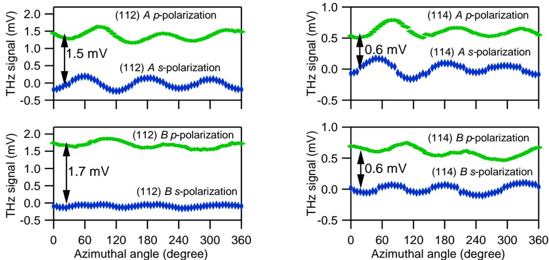
Fig. 3. Reflection geometry: Horizontal (*p*) and vertical (*s*) polarization components for GaAs (112) *A*, (112) *B*, (114) *A* and (114) *B* faces in reflection geometry. The effect of transient current has been represented in terms of an offset from the zero-line. The offsets are roughly 1.5 mV, 1.7 mV, 0.6 mV and 0.6 mV for (112) *A*, (112) *B*, (114) *A*, and (114) *B* respectively.
