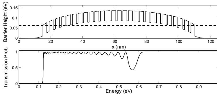
Fig. 3. The barrier shape of a mini-barrier thermionic device (top) and associated transmission probability (bottom).
