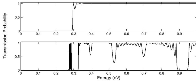
Fig. 2. Transmission probabilities for a single barrier system (top) and ten barrier system (bottom) with effective mass  $0.57m_e$  and barrier height 0.3 eV.
