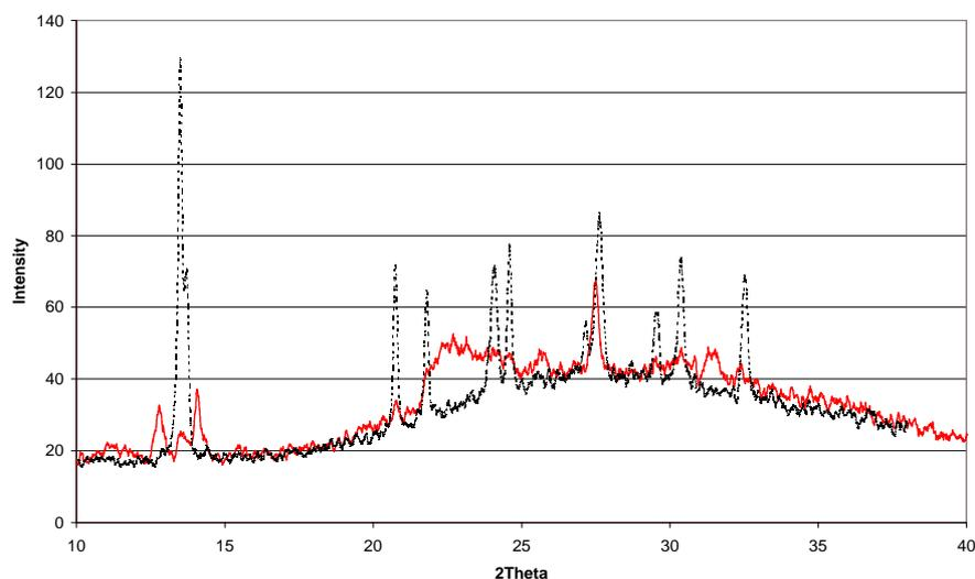
**Figure 2.** An XRD scan of a Lumogen Yellow S 0790 film deposited at room temperature (solid line) and then after being annealed at 80°C for approximately 88 hours (dashed line).
