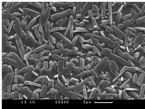
*Figure 3. SEM image of a thin film of Lumogen® Yellow S 0790 deposited on a silicon dioxide slide. The substrate is evident between the developing crystals.*
