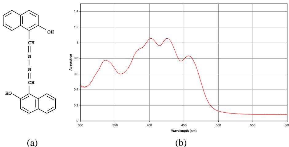
**Figure 1.** (a) The chemical structure of Lumogen® Yellow S 0790. (b) UV-vis absorption spectrum of a Lumogen Yellow S 0790 film, deposited onto a room temperature substrate. Note that the emission spectrum of lumogen ranges from 500 to 650 nm [4].
