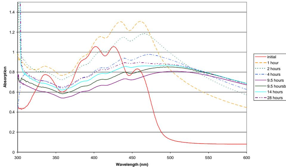
**Figure 4.** Changes in the absorption spectrum of Lumogen coating after annealing at 80°C for various time periods. The initial spectrum represents the absorption for a thin film deposited on a room temperature substrate. Note the dramatic increase in absorption at longer wavelengths after only a short period of annealing. .
