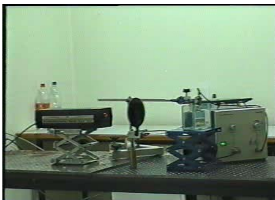
Figure 1. Experimental set-up for measuring sound speed in liquids
